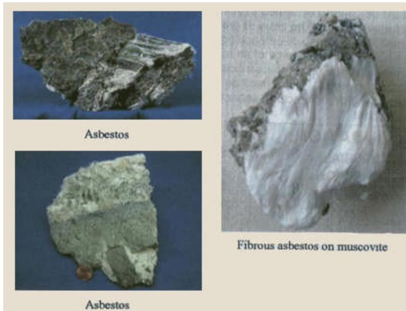
Asbestos' flexibility, heat resistance and durability make it an extremely practical product. At the height of its popularity, over 3,000 commercial products contained asbestos. Materials containing asbestos are used to fireproof, insulate, soundproof and decorate.
